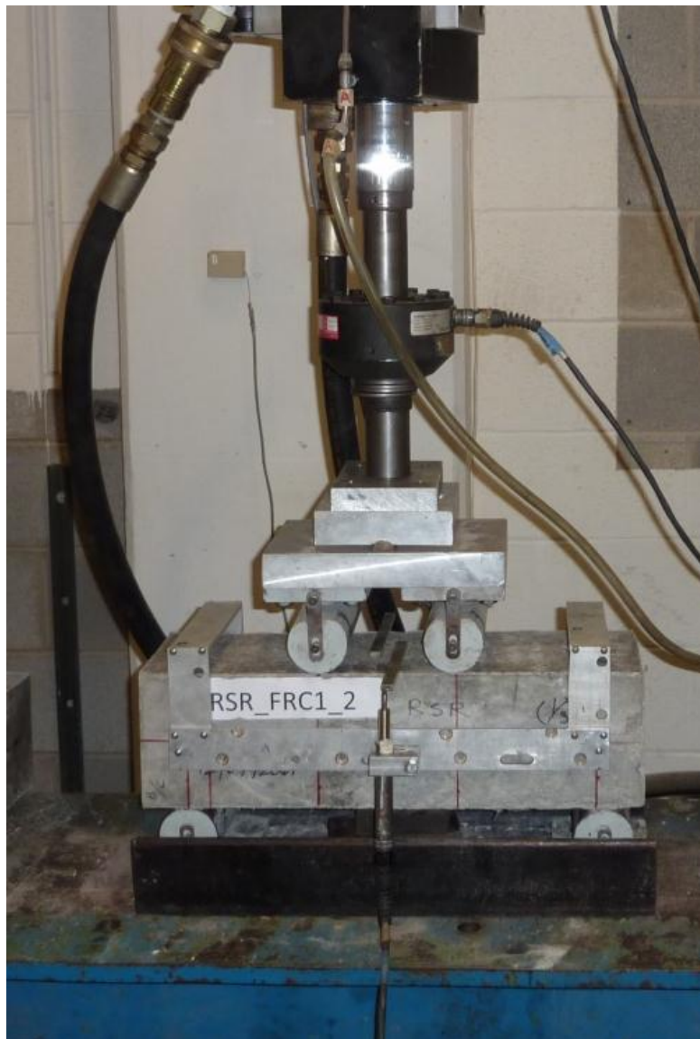
Figure 4-4: Residual strength ratio testing.
